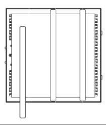
Place charcoal filter on back-side of baffle filter. And place filter brackets over charcoal filter and secure in place by tucking each end of bracket under the baffle filter frame. Re-install baffle filter.
