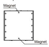
Place charcoal filters to back side of baffle filters. Secure charcoal filters in place by rubber clips. Depending on filter design secure top and bottom of charcoal filters by either rubber clips or magnets.
