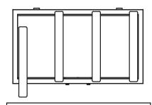
Place charcoal filter on backside of filter. And place filter brackets over charcoal filter and secure in place by tucking each end of bracket under the filter frame. Reinstall filter.
