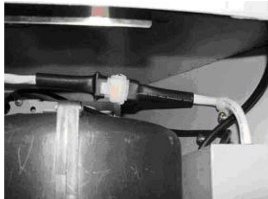
2. Connect 6 pin male connector from blower wiring to 6 pin female connector in the power pack. (plug is located inside the power pack protruding from the white control board box).
