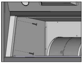
**3.** (If applicable) Remove left and right side-spacer panels by removing (2) screws from behind each panel.
