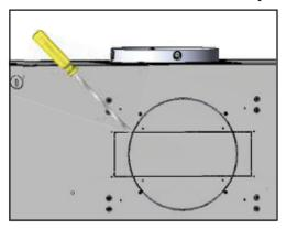
Using a flat head screwdriver, remove 8" round or 3 1/4"x10" rect. knock-out plates at the back of the liner.
