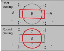
**8.** Remove knock-outs A and B for rectangular ducting. Remove knock outs B and C for round ducting.
