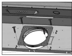
10. (Round Ducting) From inside the liner, push 8" round adaptor through the back knock-out and secure to interior back wall of liner with (4) M4 x 6mm screws.
