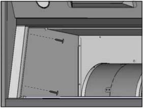
(AK9228AS Only) Remove left and right sidespacer panels by removing (2) screws from behind each panel.
