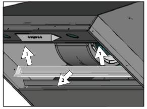
Remove grease tray by: 1) Pulling up on tray to release from bottom panel. 2) Lifting tray out of liner body.
