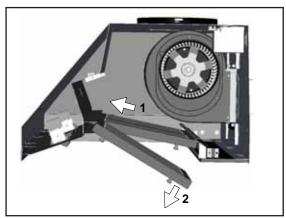
**1.** Remove baffle filters by: **1)** Pulling filter toward front of liner. **2)** Pivoting rear of filter down.
