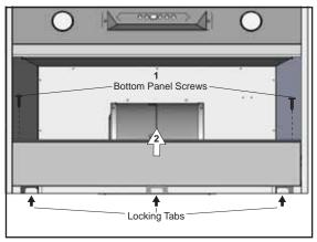
4. Remove bottom panel by: 1) Removing (2) screws from left and right sides of bottom panel.2) Pulling bottom panel toward front of liner to release from locking tabs.
