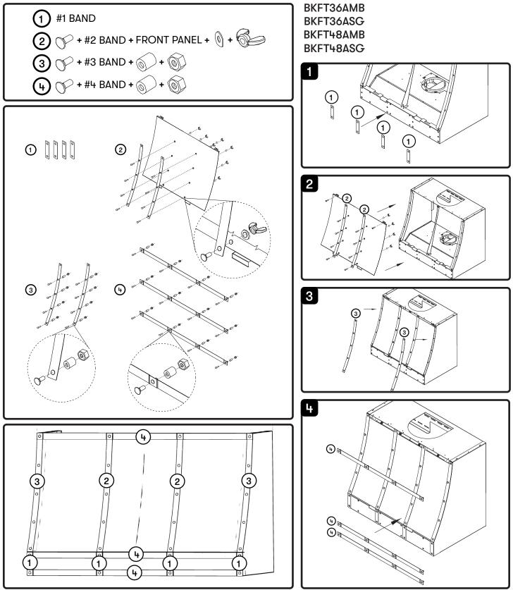
See Forte hood installation instructions for more installation details. Use the bushings, washers, and wingnuts inside the Hood Banding Hardware packet, included with the hood, to complete assembly. DEC24.0101
