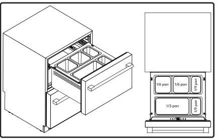
2. Install the pans into your preferred sections. The 1/9 pan must be accompanied with two 1/6 pans or one 1/3 pan for a proper fit.
