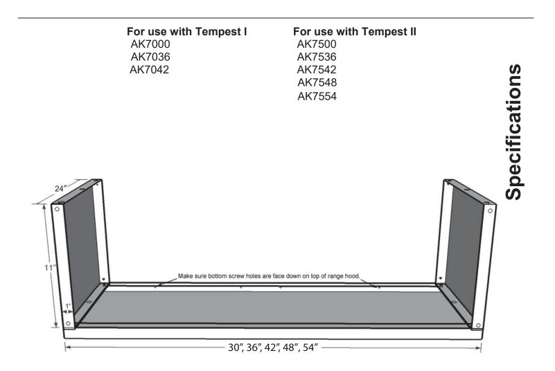
1. Line up screw holes and attach the left and right side panels to the center panel with screws provided.
