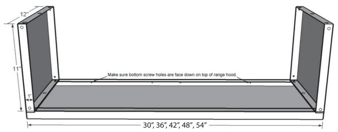
1. Line up screw holes and attach the left and right side panels to the center panel with screws provided.
