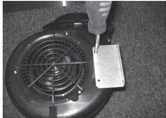
9. Attach blower brackets to blower using (2) 10x3/16" screws on each bracket.
