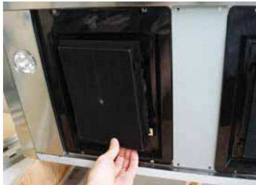
3. Install charcoal filters into charcoal filter brackets
